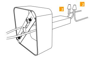
Remove backplate from canopy face and install onto the junction box. Ensure screw points for the canopy mounting are aligned properly for installation on the rail.
